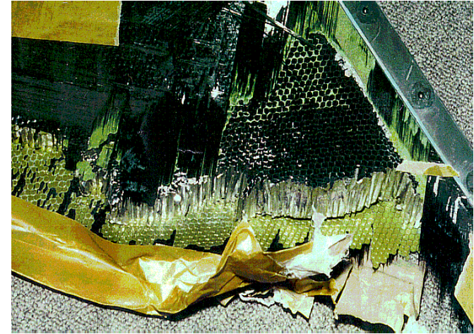
Interfacial Failure on F/A-18 Rudder
